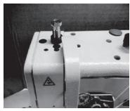
Pressure force can be adjusted simply and certainly with thumb screw at top.
