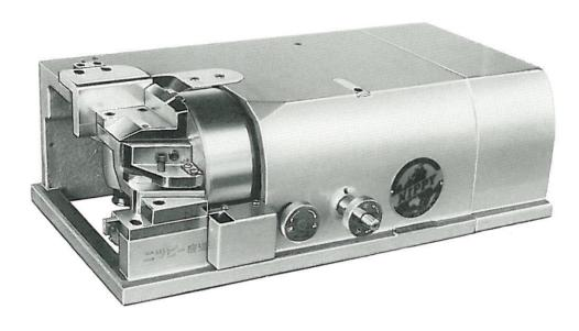
This machine skives those portions of all kinds of bag and pouch handles that protrude during the production process of sewing machine operation.
